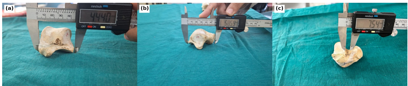
Figure 1. Representative measurement technique for dry human tali using a digital Vernier caliper
